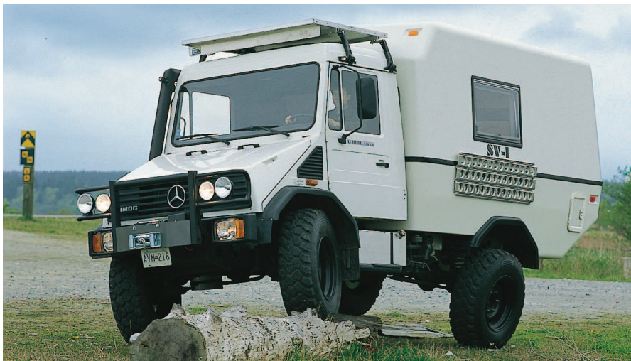
Extreme conditions are daily fare for this expedition vehicle, based on a U 100 L turbo chassis
